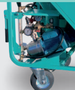
New placement of the water pump and hydraulic components designed to improve water drainage in winter. Self-priming electric pump of generous dimensions, capable of 4.5 bar of pressure. No blocking due to oxidation, thanks to the stainless steel cap and brass impeller.
