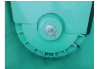
New feeding wheel design with larger cells to improve the collection of fiber materials.
