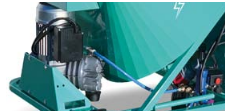
Diaphragm compressor fixed on the machine.
