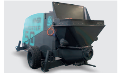
Large 350 l hopper with internal agitator.
