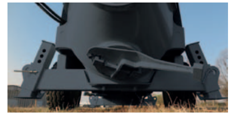
Hopper unloading door.
