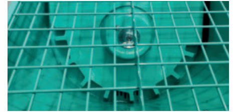
New feeding wheel design with larger cells to improve the collection of fiber materials.
