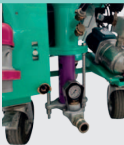
Cast iron material delivery manifold with pressure gauge. Direct connection for Ø35 F hose. It allows to extend the hoses up to 50 m, reducing wear to the stator-rotor group to a minimum. The reduction to apply the Ø 25 hose is included in the standard equipment.
